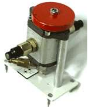
One of the hydraulic power units
