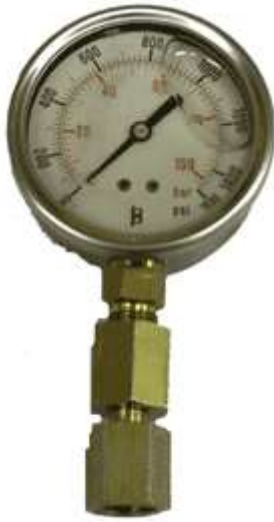
One of the hydraulic pressure gauges
