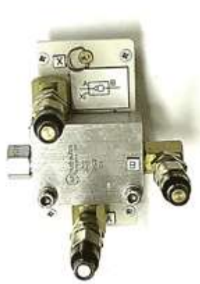
One of the piloted check valves
