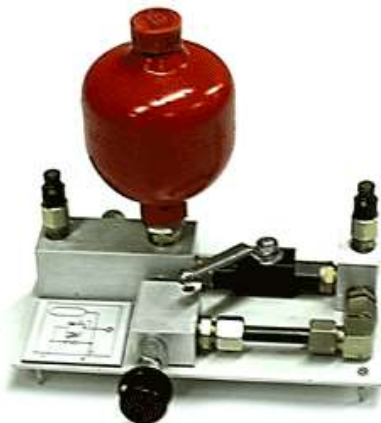
One of the hydraulic accumulator blocks
