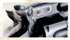
The sturdy, stirrup-style top latch on the second model revolver ensures a firm lock for the Top Break design.
