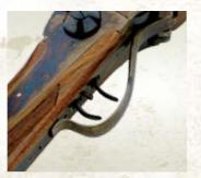
All models of Uberti's 1874 Sharps rifles, excluding the Cavalry Carbine, feature double set-triggers, allowing the front trigger to be set to a very light pull-weight—an aid to accurate shooting.
