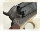
The Walker's large capacity cylinder allows it to hold up to 60 grains of black powder and offers easy access to the percussion caps.
